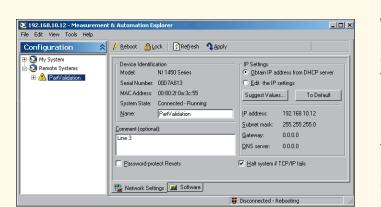
While the NI 1450 is rebooting, an 🔥 icon appears next to the device name to indicate that the NI 1450 is disconnected.
