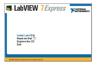
B. Insert the LabVIEW Real-Time CD. When the installation splash screen appears, click Install LabVIEW Real-Time and follow the setup instructions.
