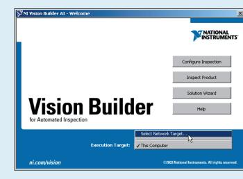
B. In the Select Remote Target window, click 192.168.10.12 to highlight the row. This IP address is assigned to all unconfigured NI 1450s.
