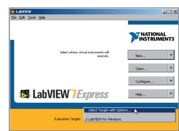
B. Type the NI 1450 IP address in the Machine Name/IP field and click OK. The NI 1450 IP address now appears in the LabVIEW Execution Target pull-down
